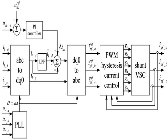
Fig.2.4 control block diagram for the shunt VSC.
