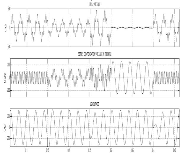
Fig.4.2 BUS2 voltage, series compensating voltage, and load voltage in Feeder2.
