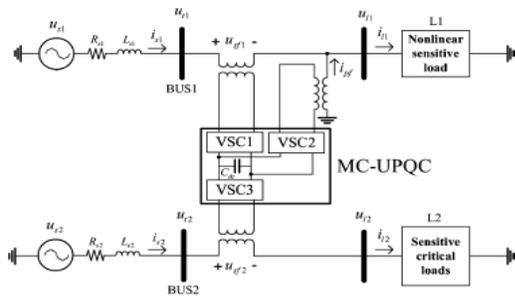
Fig.2.2 Typical MC-UPQC used in a distribution system.
