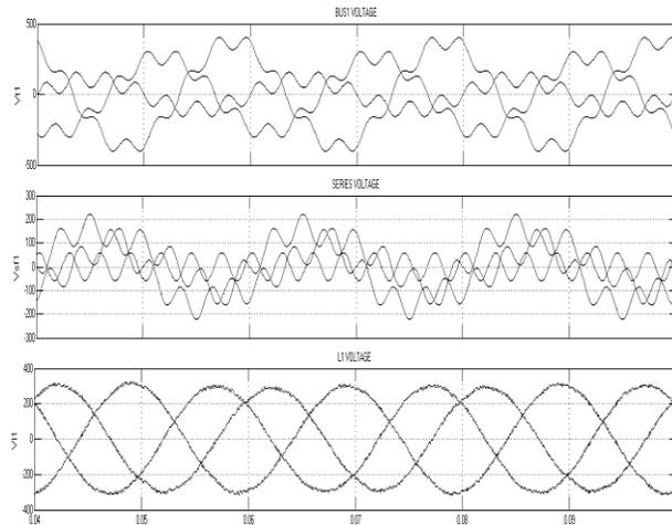
Fig.4.6 BUS1 voltage, series compensating voltage, and load voltage in Feeder1 under unbalanced source voltage.
