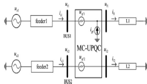
Fig.2.1 Single-line diagram of a distribution system with an MC-UPQC.
