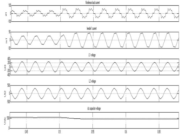
Fig.4.5 Load change: nonlinear load current, Feeder1 current, load L1 voltage, load L2 voltage, and dc-link capacitor voltage.
