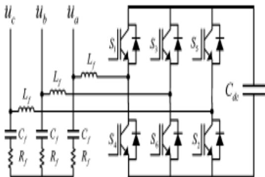
Fig.2.3 Schematic structure of a VSC.
