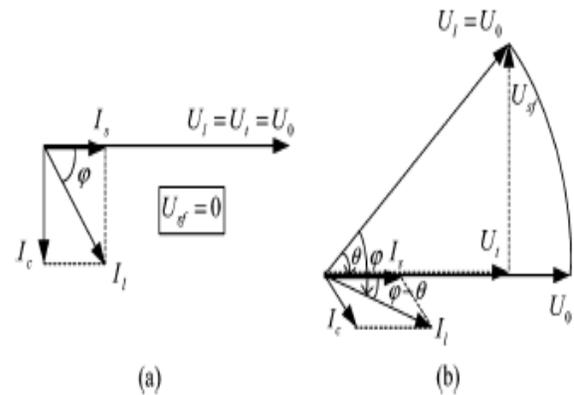
Fig.3.1 Phasor diagram of quadrature compensation. (a) Without voltage sag. (b) With voltage sag.
