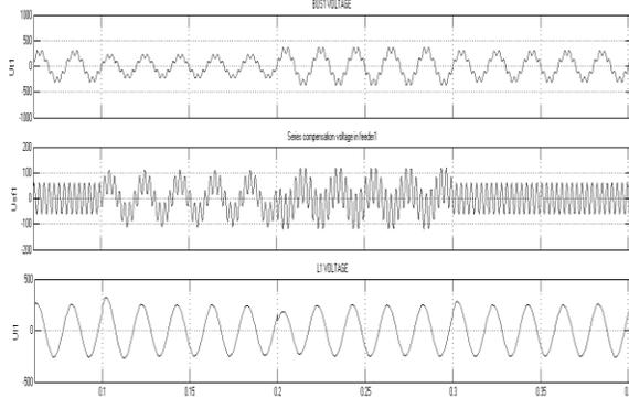
Fig.4.1 BUS1 voltage, series compensating voltage, and load voltage in Feeder1.
