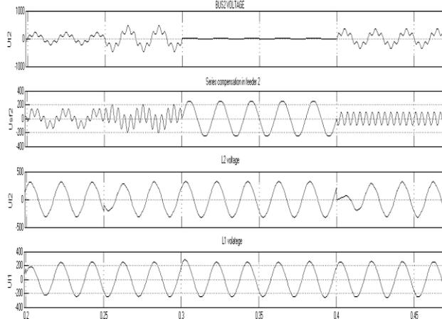
Fig.8.4 An upstream fault on Feeder2: BUS2 voltage, compensating voltage, and loads L1 and L2 voltages.
