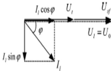
Fig.3.2 Phasor diagram of inphase compensation (supply voltage sag).
