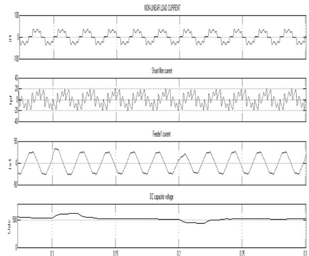
Fig.4.3 Nonlinear load current, compensating current, Feeder1 current, and capacitor voltage.
