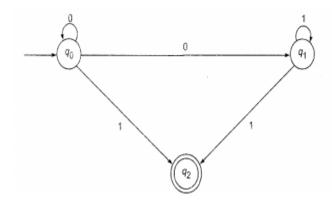
Given diagram shows the NDFA. If the automaton is in a state  $\{q_a\}$  and the input symbol is 0, what will be the next state? From the figure it is clear that the next state will be either  $\{q_o\}$  or  $\{q_j\}$ . Thus some moves of the machine cannot be determined uniquely by the input symbol and the present state. Such machines are called nondeterministic automata  $^{[6]}$
