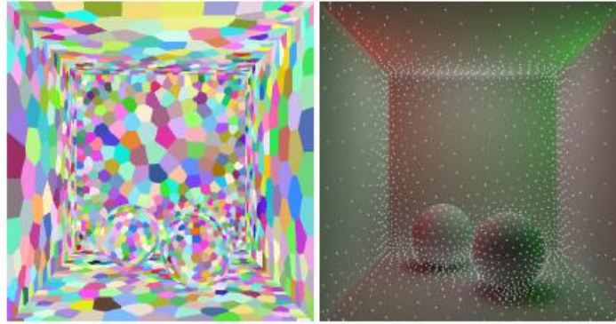
Figure 3: (a) shows our clustering result for the Cornell box scene computed with 1600 clusters; (b) displays the cluster centers on top of a raytraced reference showing the actual irradiance values.
