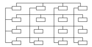
4x4 mesh Processing Elements of VLSI Processor
