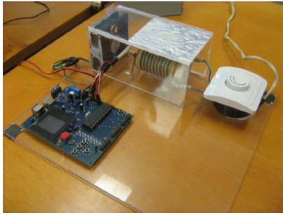
Fig. 1 – Low cost implementation of the cooling system.
