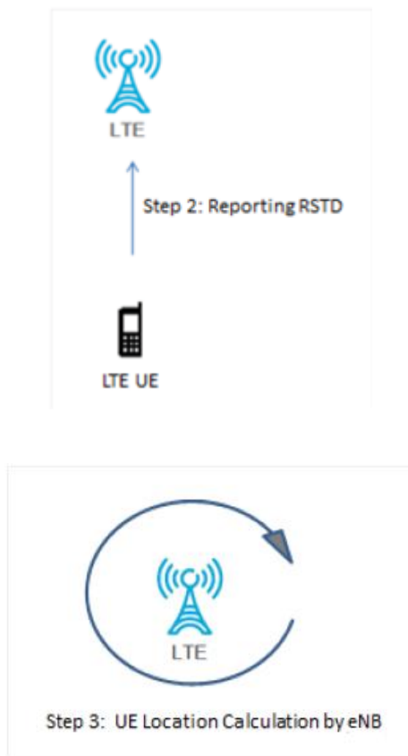
Fig 2. Process of finding UE location by using PRS
