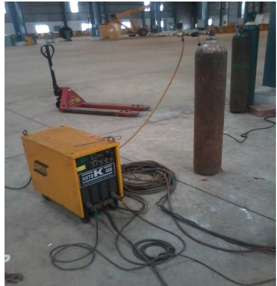
Fig.4. Experimental setup of FCAW process
