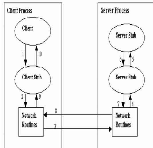
1. The customer calls the neighbourhood stub methodology. The stub bundles up the parameters into a system message. This is called marshalling.
