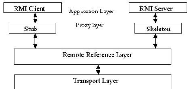
Stub/Skelton Layer: Stub/Skelton Layer is the interface in the middle of use and rest of the RMI framework. This layer does not manage specifics of transport yet transmits information to the Remote Reference Layer. A Stub for a remote-article is the customer side substitute for the remote item. A Skeleton for a remote article is a server-side substance that contains a technique that dispatches calls to the real remote item usage.
