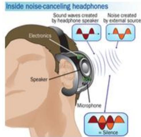
**Figure 2:** Two waves are shifted 180 degrees with respect to each other so that the waves destructively interfere. [5]
