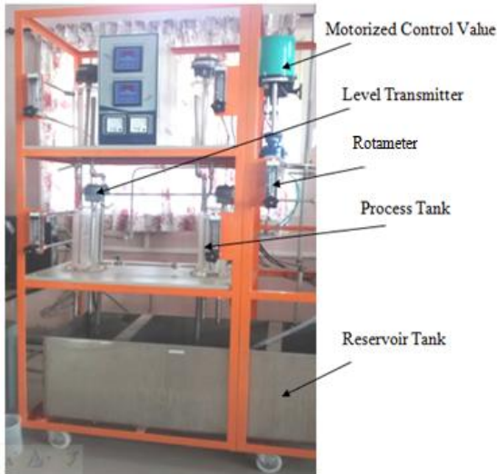
Fig. 2 Quadruple tank system setup
