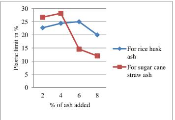
Fig 8 Comparison of plastic limit between rice husk ash and sugar cane straw ash
