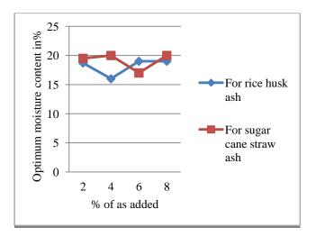
Fig 9 Comparison of OMC between rice husk ash and sugar cane straw ash
