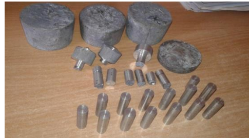
Fig 1: As cast Al-25Mg2Si-2Cu-4Mn alloy ingots and pins used for wear test
