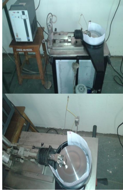
Fig 2: Pin-on-disc machine with thermocouple setup
