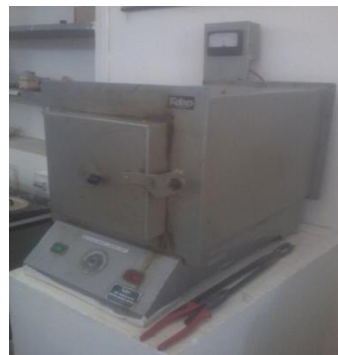
Fig 2: Muffle furnace used for heat treatment
