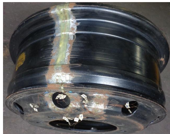
Picture showing Strain gauge located on disc For stress analysis
