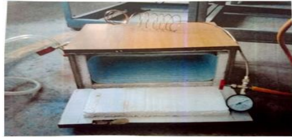
Evaporator with insulation
