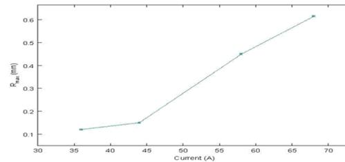
Fig 3: Rmax values with various current intensities for FEA
