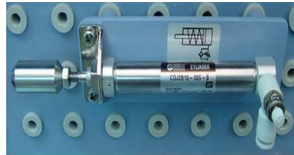
Fig. 5 (a) Single acting cylinder
