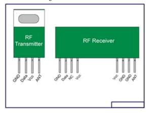
Figure 3.3: RF transmitter and receiver
