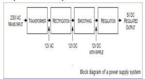
Figure 3.4: Generation of power supply Transformer – steps down high voltage AC mains to low voltage AC. Rectifier- converts AC to DC but the DC output is varying. Smoothing- smoothness the DC from varying greatly to a small ripple. Regulatoreliminates ripple by setting DC output to a fixed
