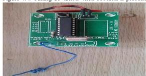
Figure 4.5: RF transmitter
