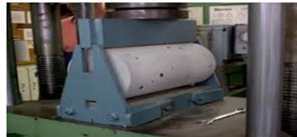
Fig:-Split Tensile Test for Cylinders
