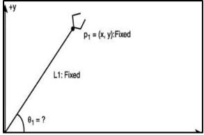
Figure 8 one link forward kinematics X=L1cos $\theta$ Y=L1sin $\theta$ [T]= $\begin{bmatrix} L1cos\theta & 0\\ 0 & L1sin\theta \end{bmatrix}$
