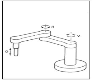
Figure 7 SCARA robots
