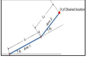
Figure 9 two link forward kinematics
