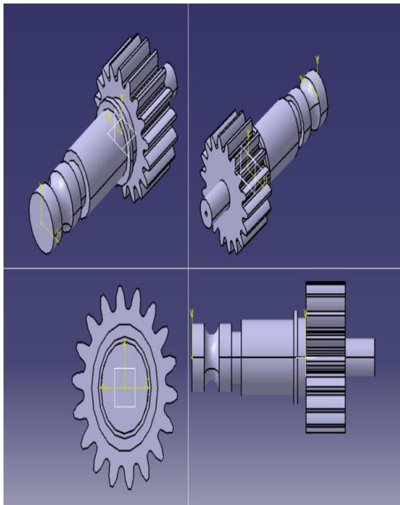
Pinion with 18 teeth is shown in the above figure. Pinion and shaft is made one piece. Shaft on the pinion is splined to ensure good grip in between pinion and universal joint.
