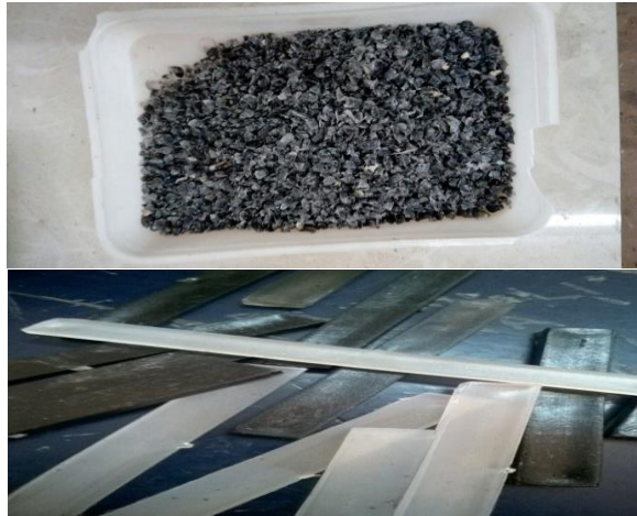
Fig.4 Fine Particles formed by grinding Fig.5 Final specimens of some compositions
