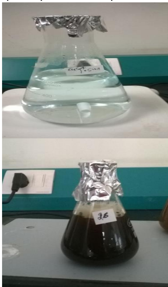
Figure: 1(a) Copper sulphate solution, (b) Cu NPs synthesized using Gymnema sylvestre
