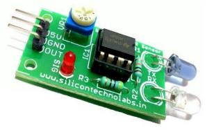
Figure 3: Infra-Red(IR) Sensors
