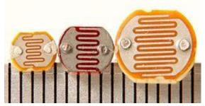
Figure: Photo Resistors
