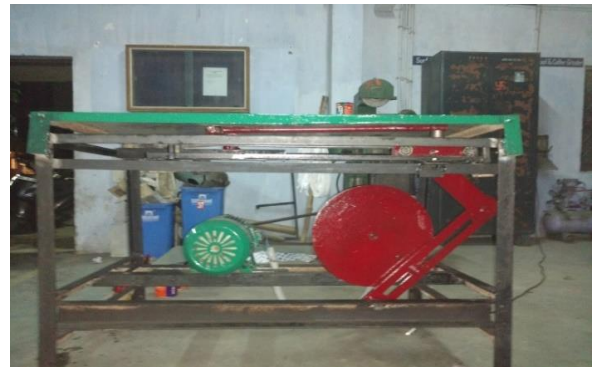
Fig. Bar Bending machine setup
