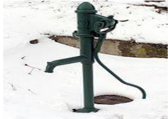
A lobe pump Hand-operated, reciprocating, positive displacement, water pump in Košice-Ľahanovce, Slovakia (walking beam pump).
