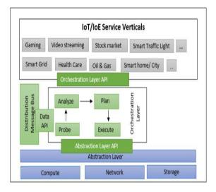
FIGURE 1. Architecture and components of fog computing.
