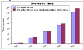
Fig. 8. The overhead of checking for deduplication on the remote site before sending the data.
