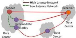
Fig. 3. The multi-route transfer schema based on intermediate cloud nodes for inter-site transfers.
