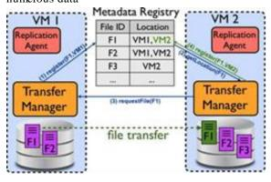
Fig. 2. Architecture of the adaptive protocolswitching file management system [6]. Operations for transferring files between VMs: upload (1), download (2,3,4).management services to process highly distributed work-flows orchestrated by multiple engines.
