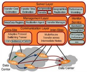
Fig. 1. The extendible, server-based architecture of the OverFlow System.
