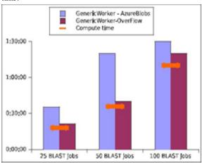
Fig. 11. The BLAST workflow makespan: the compute time is the same (marked by the horizontal line), the remaining time is the data handling.
