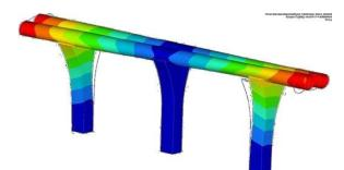
Fig. VIII. First mode shape of Hyperloop at 2.71Hz (magnified x1500)
