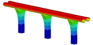
Fig. IX. Second mode shape of Hyperloop at 3.42Hz (magnified x1500)
