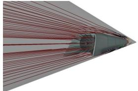
Fig. IV. Streamlines for capsule traveling at high subsonic velocities inside Hyperloop.
