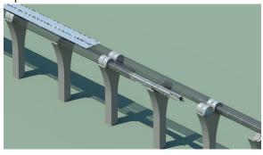
Fig. X. Hyperloop capsule in tube cutaway with attached solar arrays
