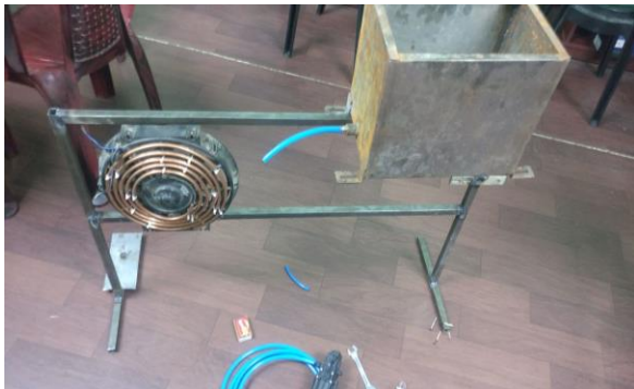
FABRICATION OF AIR COOLING SYSTEM
