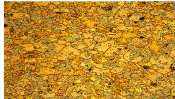
Figure 3.4: Micrograph of MMC (Al 356 alloy with reinforcement).
