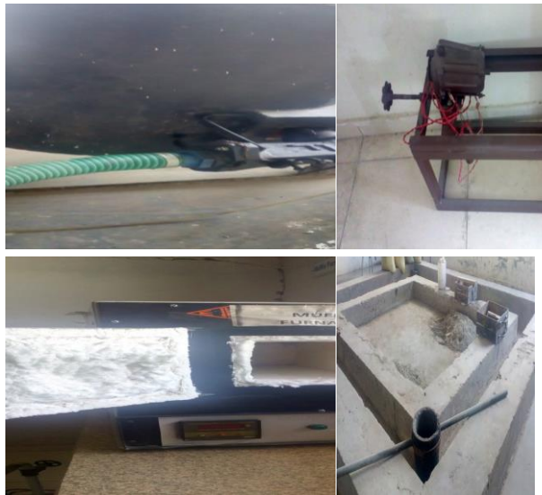
Figure 3.1: Stir Casting Set Up.
