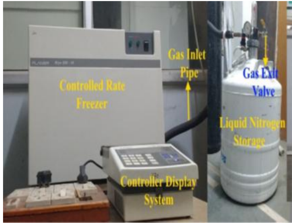
Fig.1.2: Set up for cryogenic treatment of the tool electrode.
