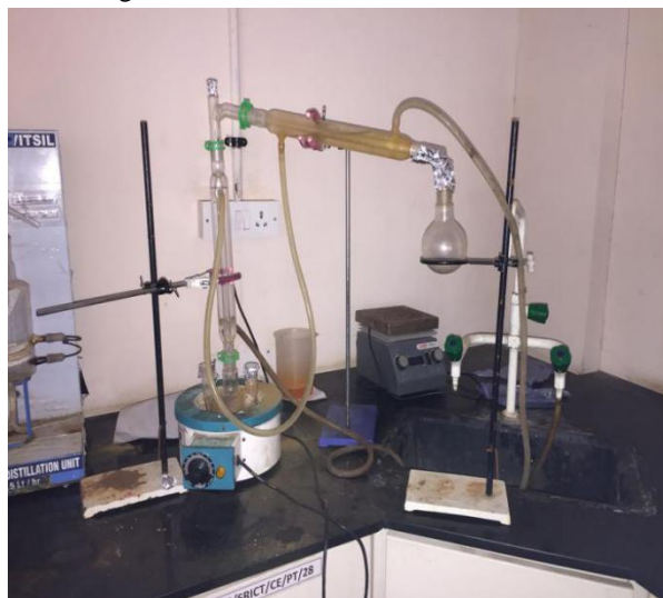
Figure 2.2.1 Refluxed of adsorbent with alkali water
