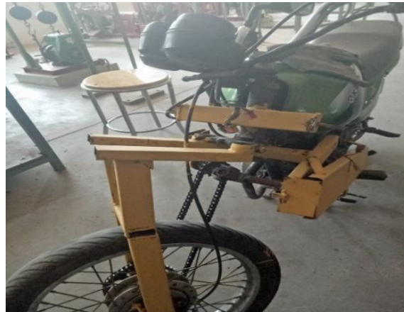
Fig.4 Front wheel driving Mechanism
