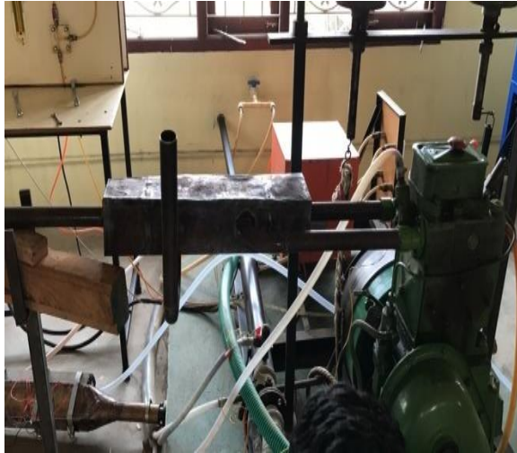
Fig 8: The Pre-Heating Chamber Set Up on the Diesel Engine
