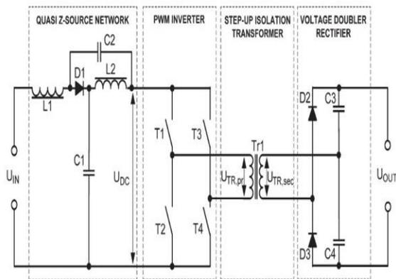
Figure 3. Simplified power circuit diagram of the proposed converter
