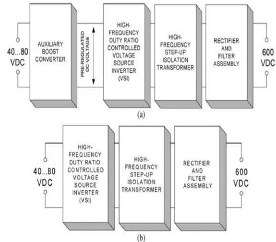
Figure 2. Generalized structures of most widespread front-end step-up isolated dc/dc converters for residential FC power systems
