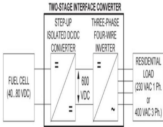
Figure 1. Typical structure of the interface converter for residential FC-powered systems
