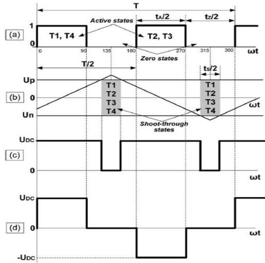
Figure 2. Proposed operating principle and resulting voltages of the single-phase qZSI in the shoot-through (voltage boost) mode
