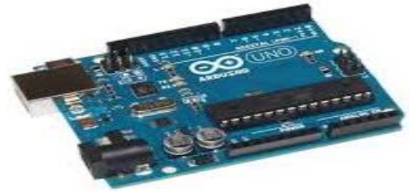
Fig. 1. Arduino uno. It controls the RFID detection tag to sensor and sends information into the server. Basic pin information on Arduino.
