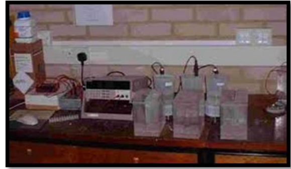
Figure3. RCPT set up
