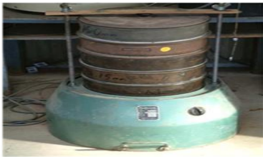
Figure - The shaking device and stack of sieves used to conduct the sieve analysis
