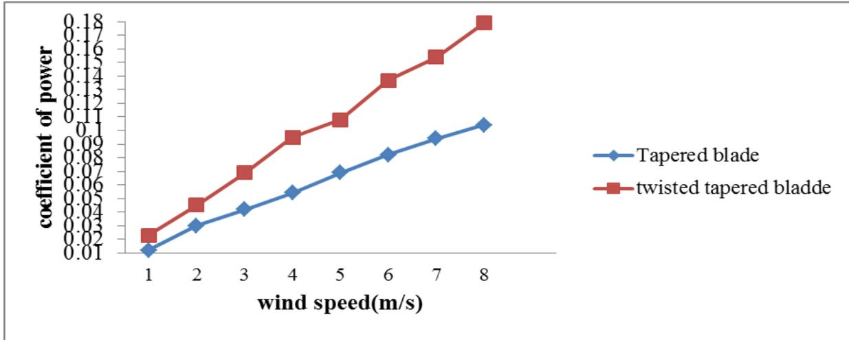
Fig 6 Variation of twisted blade and simple tapered values of coefficient of power
