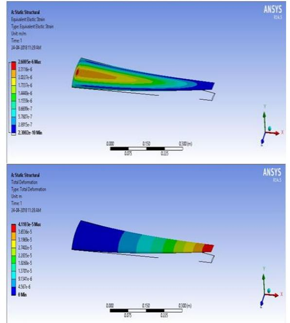
(c). Equivalent elastic strain (d). Total deformation
