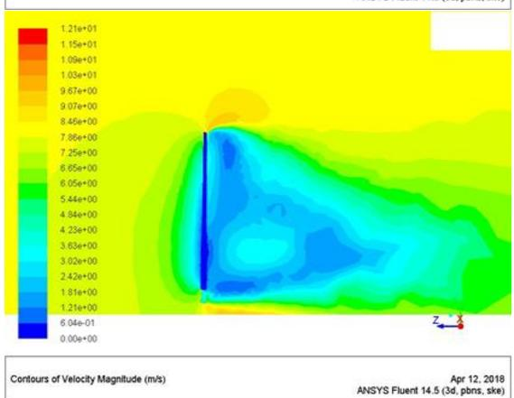
(a) Velocity contour for Simple tapered
