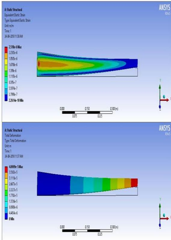
(c). Equivalent elastic strain (d). Total deformation
