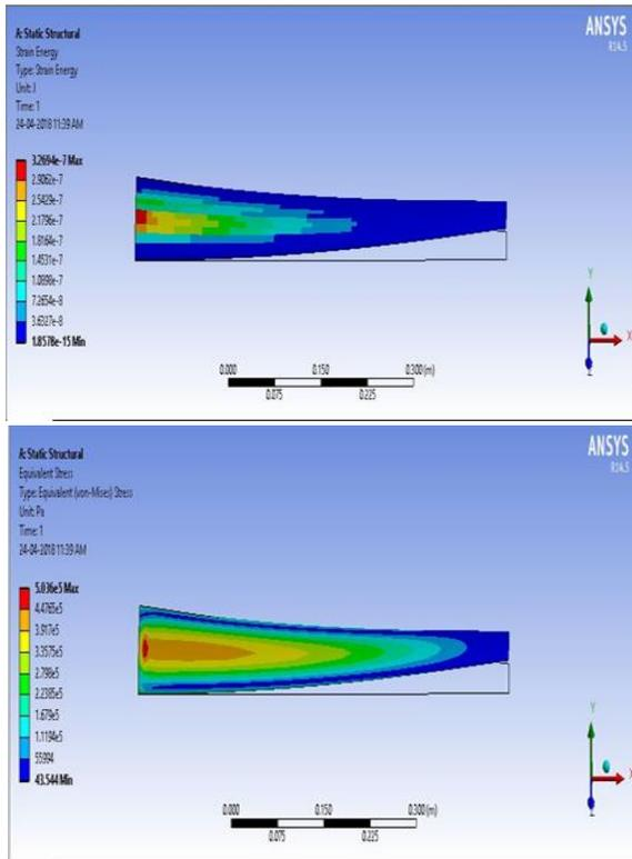
(a). Strain energy (b). Equivalent stress
