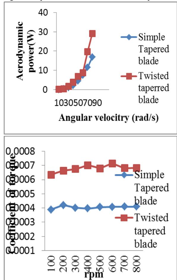
Fig 4 Variation of twisted blade and simple tapered blade value of aerodynamic power and coefficient of torque with angular velocity and rpm respectivel
