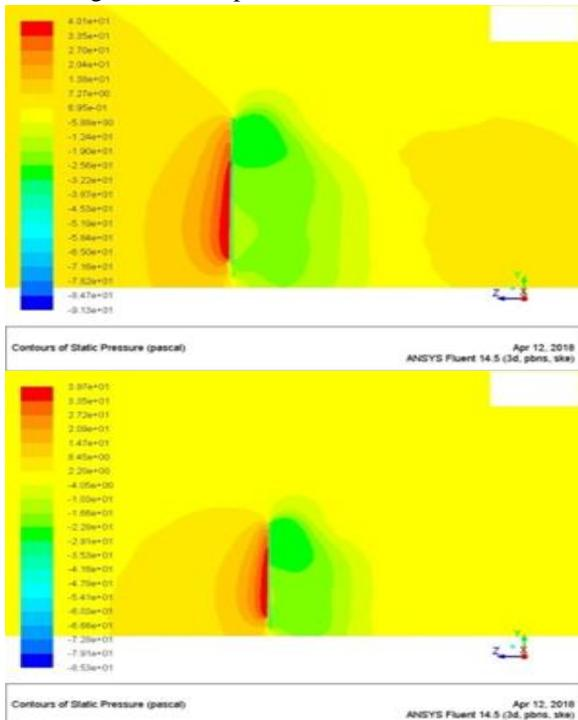
Fig 7 Pressure contour of the simple tapered and twisted tapered blade of the wind turbine at 8m/s for comparison
