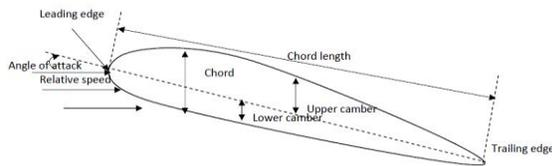
Fig 1 Basic wind turbine blade structure
