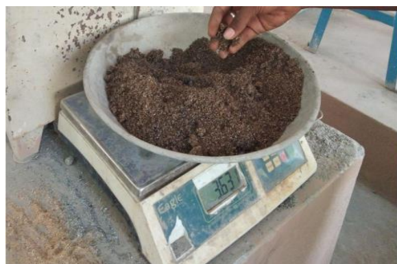
Figure 1: Steel Slag, Fine and Coarse Aggregate Steel slag is mildly alkaline, with a solution pH generally in the range of 8 to 10. However, the pH of leachate from steel slag can exceed 11, a level that can be corrosive to aluminum or galvanized steel pipes placed in direct contact with the slag
