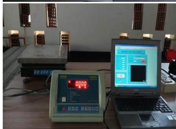
Fig3.1.5(a): Balance reader software Fig3.15(b): Full connection setup of the balance recorder
