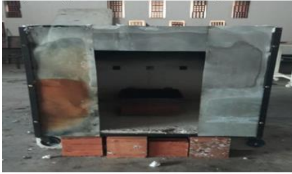
Fig: 3.2.1.(b): Flashover Apparatus setup
