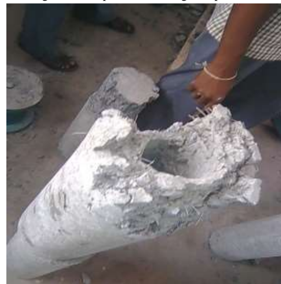
Figure 2. Failure of hollow columns under direct compression
