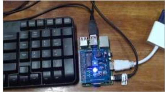
Fig 7 Result of execution of Program for LED Blinking
