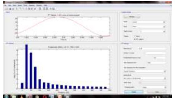
Figure 5.16 FFT analysis for inverter output voltage at mode 4
