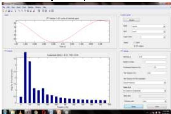
Figure 5.6 FFT analysis for inverter output voltage at mode 1
