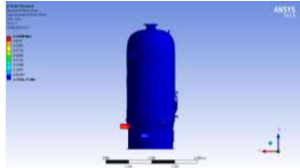
Figure 4.4 Equivalent Elastic Strain in vertical shell pressure vessel of structural steel material
