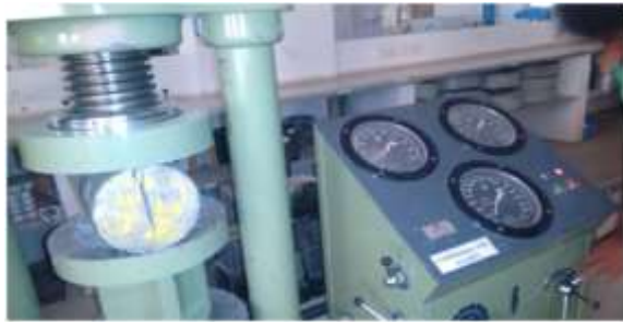
TENSILE STRENGTH TEST RESULTS FOR 7 AND 28 DAYS
