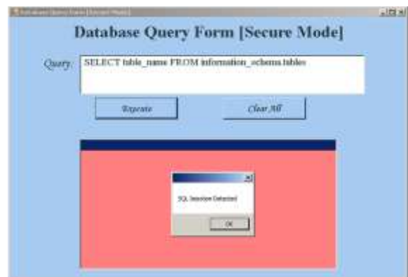
Fig. 12 Secure Mode: Demonstration for Case IV Case V: SQL Injection Attack pertaining to relational operator based tautology
