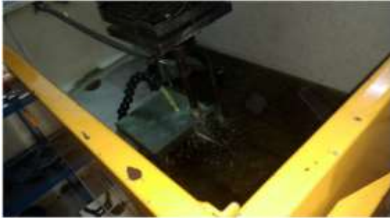
Fig: 3.2: EDM machine during machining of EN 31 steel
