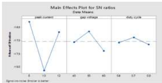
Fig. : 4.1: Main effects plot for S/N ratio for surface roughness
